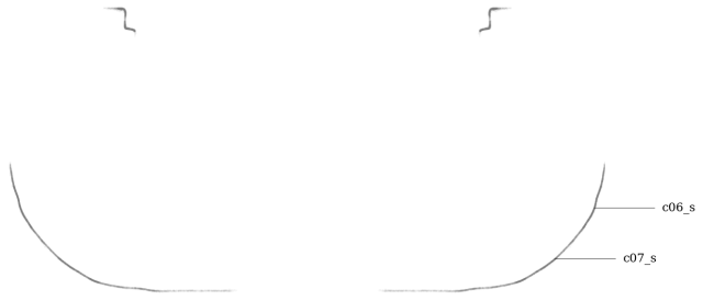
Figure 32: Circularity measurement sample location, separately aligned interior mesh
