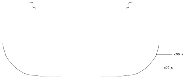
Figure 79: Circularity measurement sample location, separately aligned interior mesh
